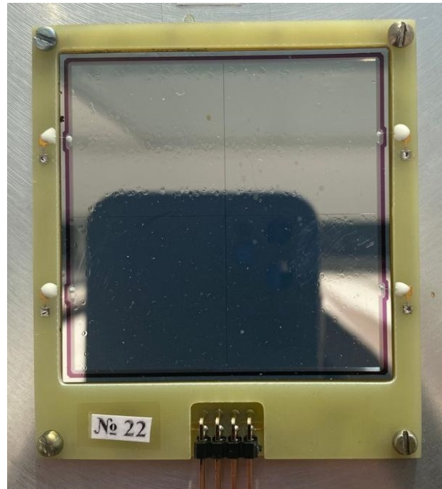
Figure 5: Silicon semiconductor detector used as a stop detector in the TOF \Delta E - E_r spectrometer.
