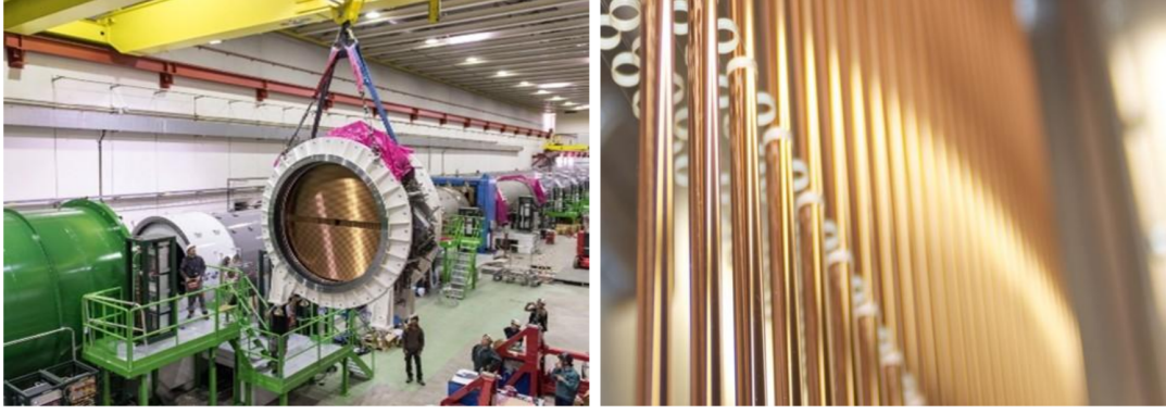
Figure 4: Left: Installation of the NA62 tracker module. Right: Photo of the NA62 tracker plane.
