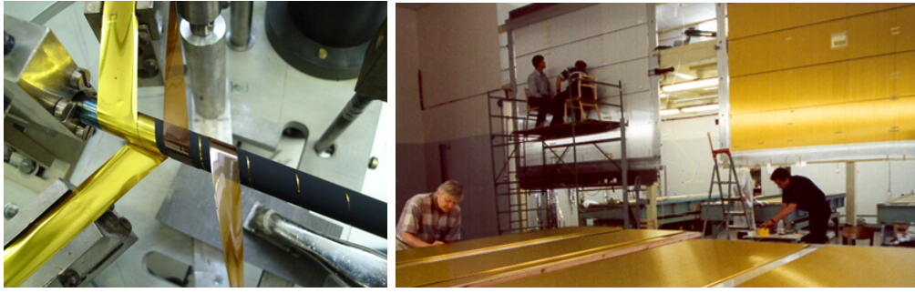
Figure 1: Left: Winded straw production. Right: Assembling of the COMPASS Straw Tracker modules.
