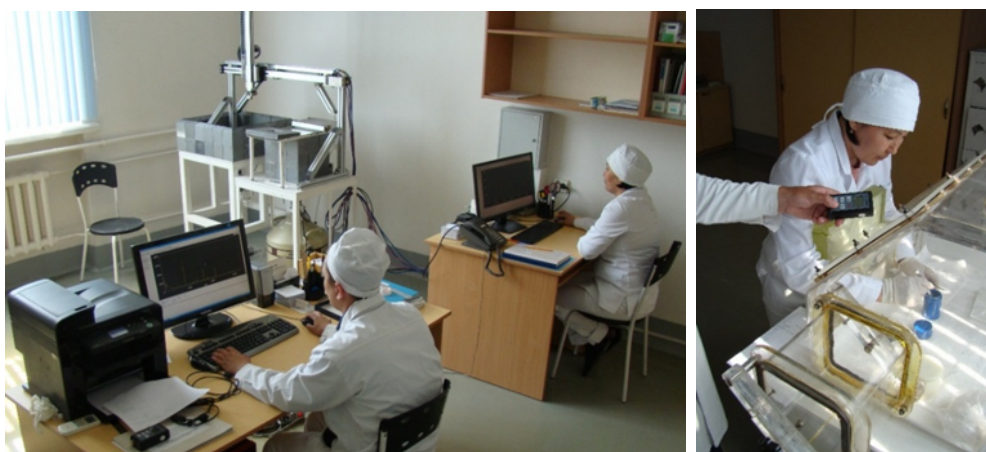
Figure 7: Automated section for conducting NAA on medium- and long-lived isotopes
