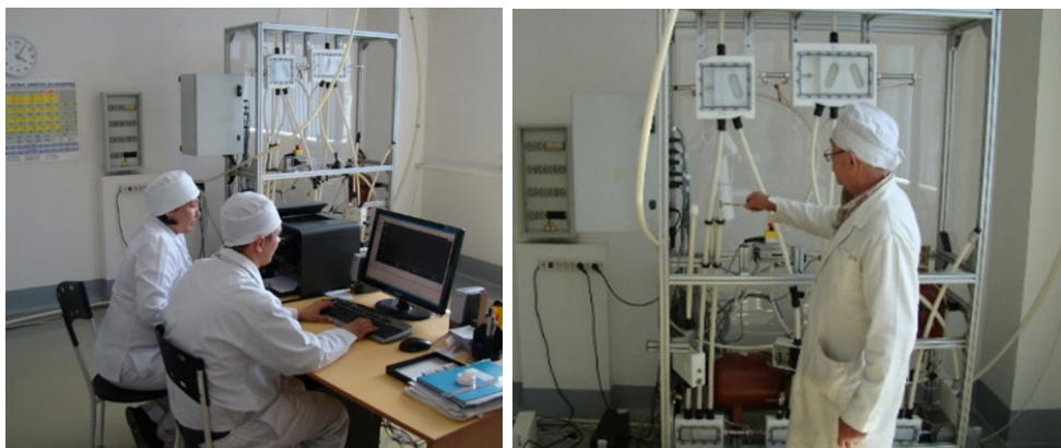
Figure 6: Pneumatic transport system for NAA for short-lived isotopes
